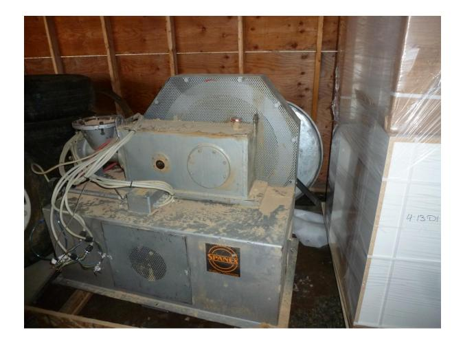
Spaenex model 394 + spare parts 150 - 180 KG per hour 11 Kw Motor 400 V 27.5A All wire, transformer
